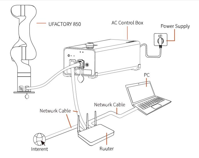
3. PC and router are connected by wireless network, and control box and router are connected by Ethernet cable. **Note:** It is not recommended because of the delay and packet loss of wireless connection.
