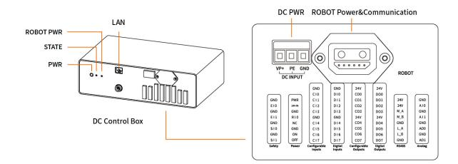
**ROBOT PWR:** The power of robotic arm, it will be RED after enabling the robotic arm. **STATE:** The state of controller, it will be GREEN after powering on the controller. **PWR:** For internal debug only.
