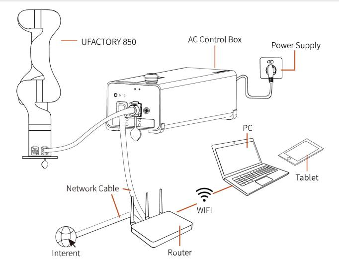
4. The control box, PC and network switch are connected by Ethernet cable.
