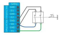
This configuration is only for applications where the operator is unable to close the door from behind. Configurable I/O can be used to set the reset button outside the door, as to reactivate the movement of the robotic arm. Another example of an automatic recovery is the use of a safety pad or a safety laser scanner, see the figure below.
