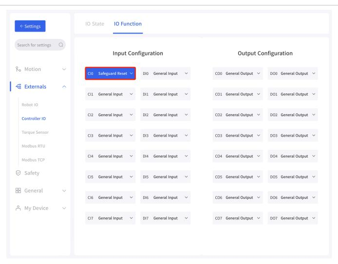
If 850 needs to resume motion, connect SIO and SI1 to GND, and trigger the motion of 850 by connecting CIO to GND; if 850 needs to pause the motion, disconnect SIO and SI1 from GND.
