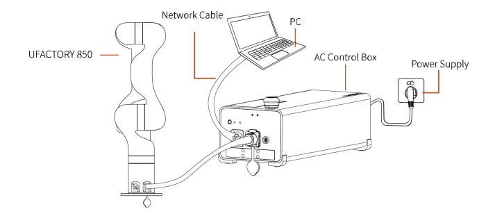
2. The control box, PC and router are connected by Ethernet cable.
