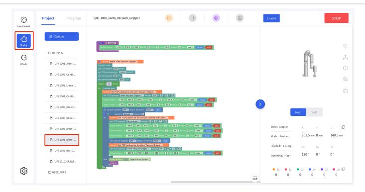
The role of this program: execute this program to control the vacuum gripper to suck the target object at the specified position, and then place the target object at the target position.
