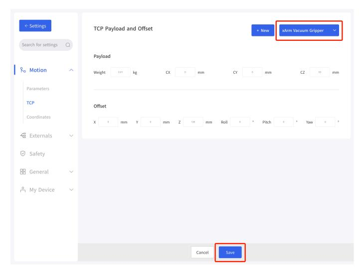
After installing the vacuum head, set the Tcp load and offset, select the 'xArm Vacuum Gripper' and remember to save it!
