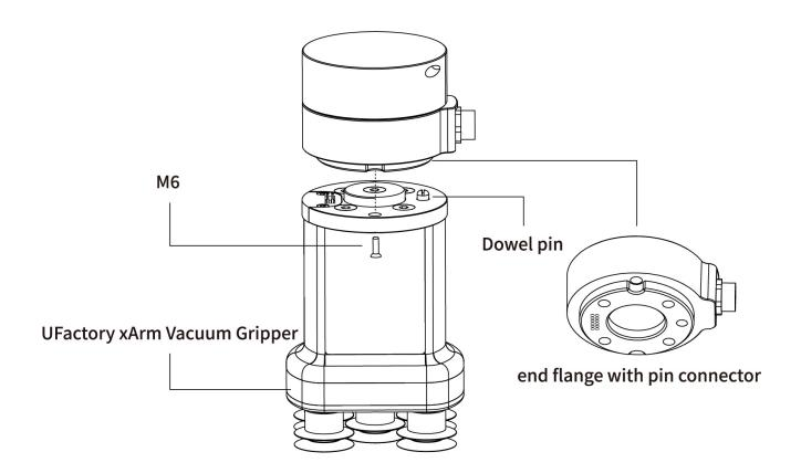
• If the end flange of the robotic is equipped without the pin connector
