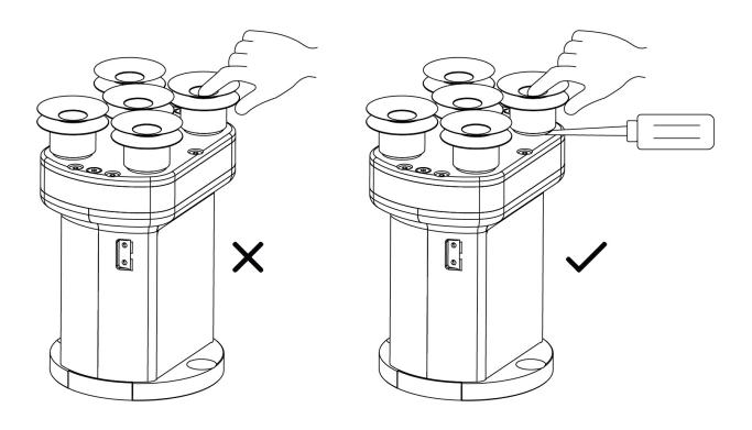
5. Please use a wrench to tighten the unused nozzle with M5 sealing plugs, to ensure air tightness.
