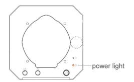
After pressing the power button, the power indicator lights up, indicating that the robotic arm is turned on.
