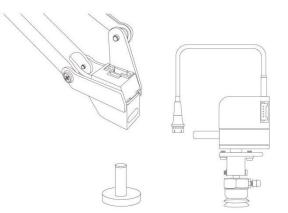
**Step 2:** Connect the wires of the fourth axis, the suction tube and the limit switch.
