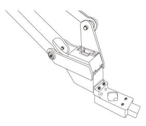
Way 2: Remove the two screws at the front of the universal penholder , connect the fourth axis motor
