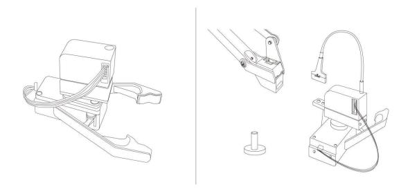
**Step 3:** Install the fourth axis motor and gripper.
