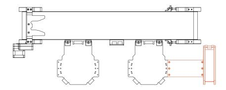
Connect the uArm Swift Pro stator to the material slide with the connection plate.
