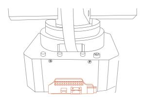
Install uArm 30P extendable base to the rear interface on uArm
