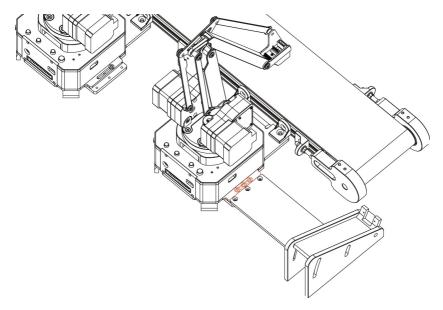
Place the Arm Swift Pro that with burnt firmware on the stator, it should stay close to the stator.
